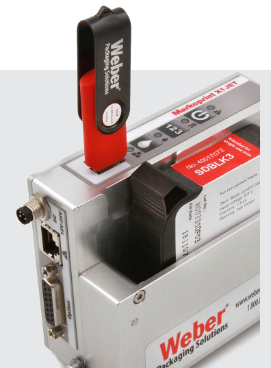
USB drive input for transfer of files created on a PC (up to 9)
